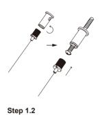
Loosen the top part of the hanging cable (C) and put the (A) screws in.
